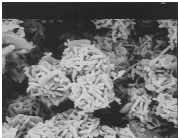
Figure 8. SEM (10 kV magnification 10 000 \times ) of clusters of plates composed of SnS + Sn obtained from the pyrolysis of (Bn_3Sn)_2S .
